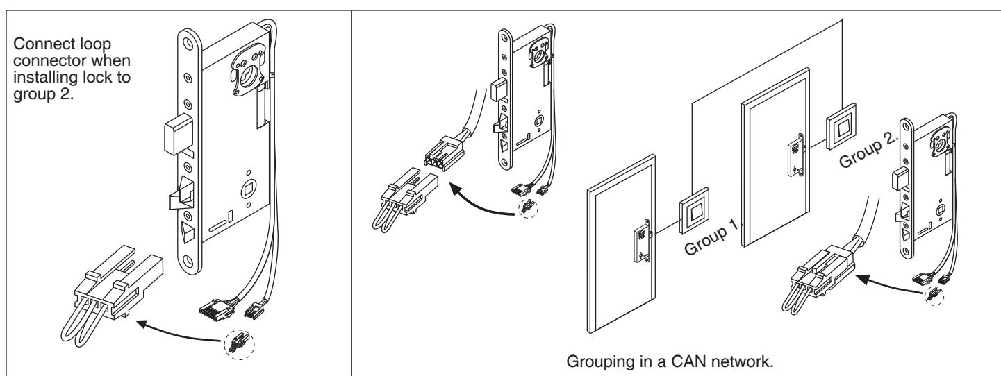
The connection to the network is accomplished by four wires, two wires for the bus network and two wires for the power supply. Please use CAN-cable ABLOY® EA216/EA226 (9 x 0,14 mm<sup>2</sup>) with the lock.
