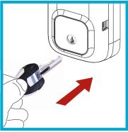
1. Insert the key into bottom of the keyway, leave the key there. Note! Don't turn the key.
